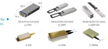
iTLA, CDM, and ICR. The integrated solution combines the units mentioned above into integrated devices including transmit-receive optical sub-assembly (TROSA) that can be an integration of iTLA+CDM+ICR or CDM+ICR, and multi-chip module (MCM) that can be an integration of CDM+ICR+DSP. Different material technologies are applicable to different packaging forms. MCM has high integration and high performance, but it requires optical chips to support non-hermetic packaging.
