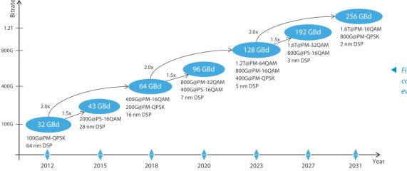
Fig. 1. Coherent optical communications evolution map.
