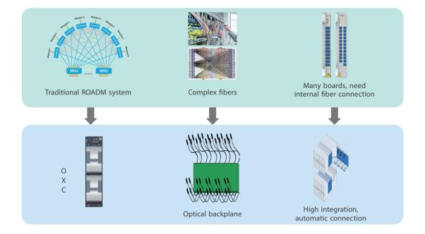
Fig. 1. Comparison between ROADM and OXC.
